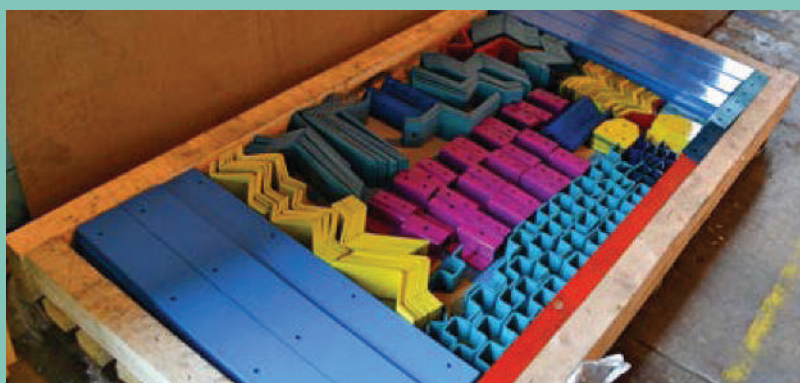
A crate of coloured brackets and fixing connections, which match to coloured stickers positioned on the components during the manufacturing process.
