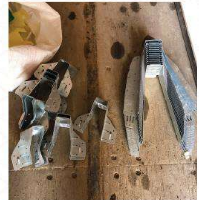
Joist hangers (14 x £3.11 each = £43.54)
