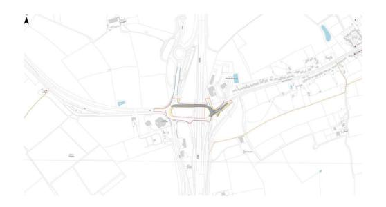
A1(M) junction 53 Scotch Corner is an existing grade-separated junction on the A1(M) to the south of Darlington. The signalled roundabout junction serves the A1(M), the A66 and the A6055 and provides access to Scotch Corner Motorway Service Area.
