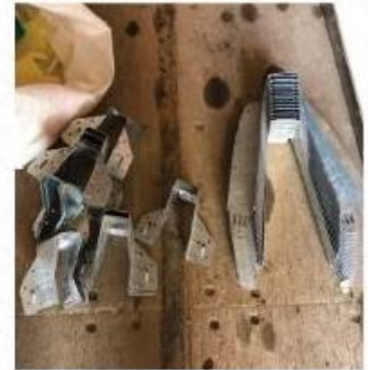
Joist hangers (14 x £3.11 each = £43.54)
