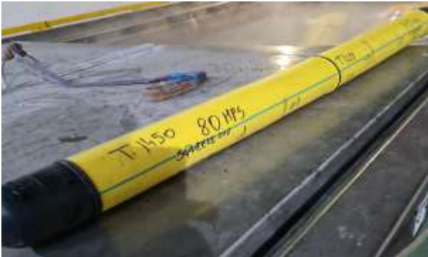
New H Pipeline (PE80 Yellow with Blue stripes)
